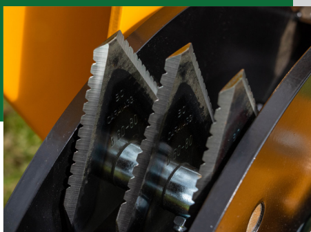
6 Reversible Shredder Knives
